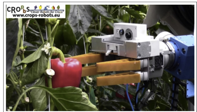
Fig. 9 – The cRops gripper and manipulator, shown here with the sensory rig that includes both RGB and range cameras. Registration was done in software and provided RGB-D point cloud used for the analyses and experimental evaluations discussed in this paper.
